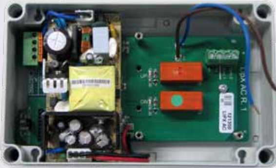
Flex1 ACDC as supply for motors with own overload protector. (Chain & Rack Drives) Box size (LxWxH): 180 x 110 x 63 mm
