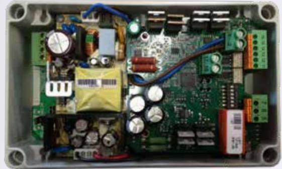
Flex1 ACDC as supply for build in overload protector ex. LIP7 OC #121308 Box size (LxWxH): 180 x 110 x 63 mm
